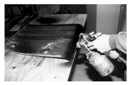
10. Take the new floor panel and flip it over. Remove all traces of oil with thinner and spray a coat of black Krylon or DP90 black around the edge. This will make the final scribe mark stand right out. Let it dry for ten minutes.
