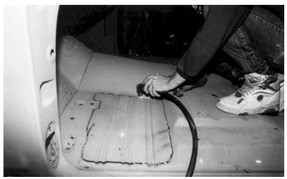
2. Take a plasma cutter like this Hypertherm MAX 20 and cut one inch below the scribe mark, as seen.(or use a cut off tool with a 3/32 wheel) This is just to get some of the metal out of your way so the new floor will fit down into place, giving you a better final fit. You can also use an Ingersol Rand cut off tool with a 3/32 grinding wheel to cut the floor if you are on a budget.
