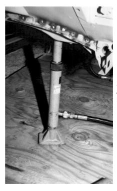
20. Take a Porta Power and press against the floor brace to make it tight up against the floor. Use a block of wood between the Porta Power and the brace. If your on a budget, use a floor jack with a 2 X 4.
