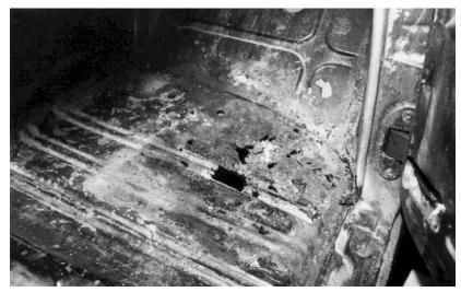
This photo shows a typical rusted out floor panel on a 55,56,or 57 Chevrolet. Although the following technique will work with any floor pan.
