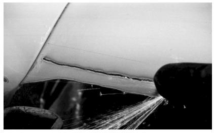
8. Remove the new floor pan and cut about a 1/2 inch below where you scribed your line on the cars existing metal.
