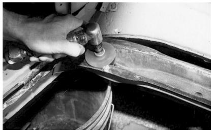
5. Take an Ingersol Rand 302 angle grinder and grind down all the welds that were left behind from cutting the floor free from the brace. A Mirka Trim Kut disc works well to grind them smooth.
