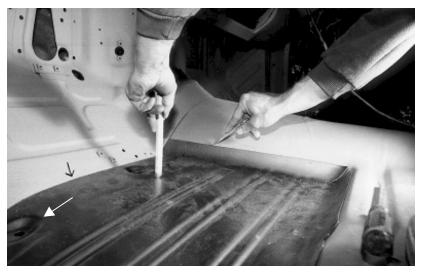
7. Lay down the new floor panel, and take a round punch and line up the floor brace to the hole in the floor pan where the bolts went through, Then install a new bolt through the hole in the new floor towards the rocker. Tighten it down. See white arrow. This will pull the floor down tight for a better fit. Run a scribe completely around the perimeter edge leaving a nice line.
