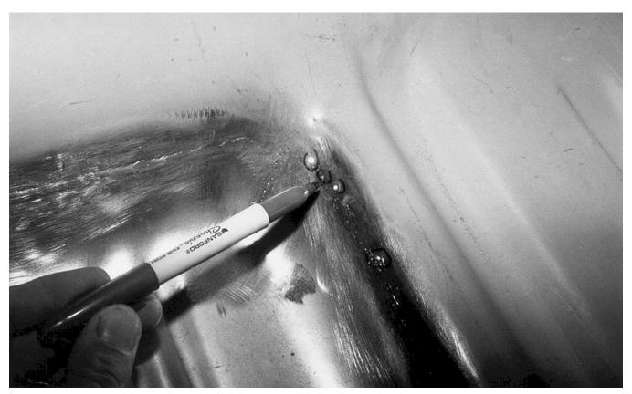
23. Now check for pin holes, by turning off all lights in the shop . Place one strong light under the panel. Any light shining through indicates areas that need to be welded. Mark a circle around these and repeat the welding and grinding steps. Finish all welds with 120 grit grind disc for extra smooth metal work.
