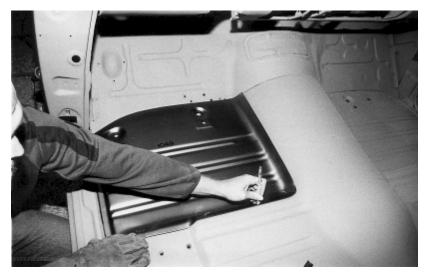
1. We started by setting a new reproduction floor panel from C.A.R.S. Inc. (800 521-2194) on top of the old piece. Line up the floor brace holes to the top of the existing body bolts. Take a carbide scribe from A and I Supply and scribe on the outside edge leaving a nice line. 25 PHOTOS
