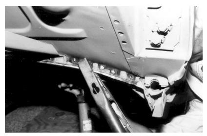
19. The seam needs to be welded where the floor and toe panel meet.
