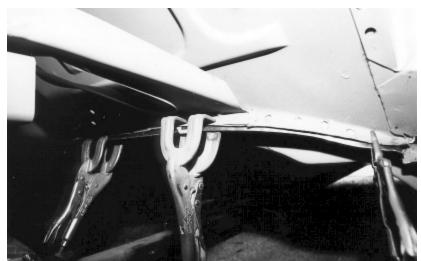
11. Re-install the floor as in step 7. Clamp the edges below the firewall, make sure the edge of the floor inside the interior is flush with the toe panel where your toes would rest as seen in Photo: #7.
