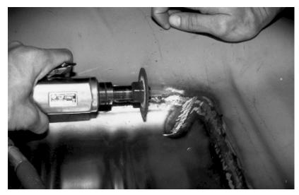
22. Grind the welds with a Cut Off tool using a 3/32 wheel for optimum results.
