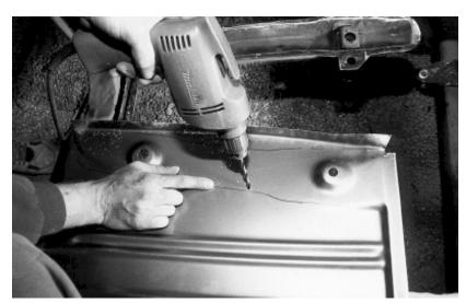
16.The floor brace is 1/2 wide. So measure 1/4 from the marker line drawn in step 12 toward the inside brace. This will assure centered brace holes for welding the floor to the brace. Drill a 1/4 hole every two inches.
