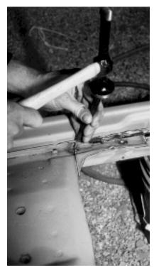
4. Drill out or plasma cut the spot welds where the outside rocker meets the floor. Then take a chisel and a hammer and separate the metal from the rocker panel edge.
