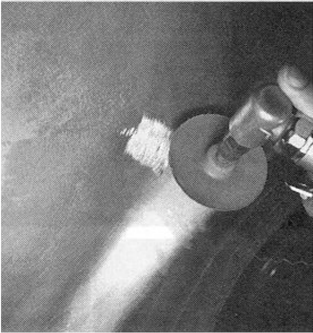
15. The welds are ground down with an angle grinder, cleaned, and dressed with the dual action or orbital sander.
