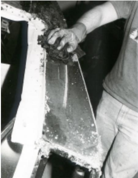
10. As seen in this top view of the quarter panel, you should wash down the stripped panels with lacquer thinner and a clean cloth. This will remove small remnants of the acid stripper and paint residue. The cleaner it is, the better the adhesion will be later. 3M Scotch Brite scuff pads #7447 will speed up this process considerably if your not on budget restraints!
