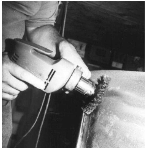
12. Now that the paint has been all removed with the Klean strip you must clean up the steel and any remnants of paint or body filler left. Use a sander with 36-Grit Disc. This is the most efficient way for cleaning up the paint remnants and old body filler.
