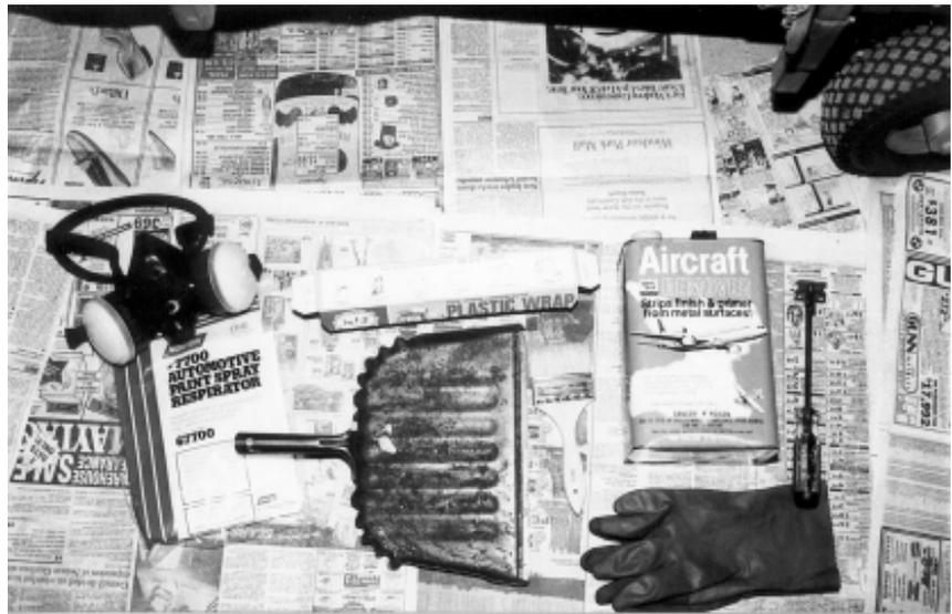
4. Take the can and pour a nice trail of the stripper over the area you are working. An alternative method is to take a container which will not be melted by the acid and fill with stripper for easier dispensing. NOTE1 This product will burn your skin if contact is made! Keep a bucket of water nearby for quick rinse if it touches your skin, this will take care of it. Keep your clothing and shoes out of it also. Put down more news paper on floor if needed.
