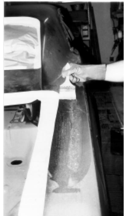
5. Use a wide brush by Marson or a 3- 5 inch hardware paint brush made for chemicals such as horse hair and dip the brush into the bowl for the needed amount, stroke the panel lightly leaving a 1/16 inch layer of the stripper. If you push down too hard the paint will roll up under your brush and you will be pushing it around rather than laying out an effective coat.
