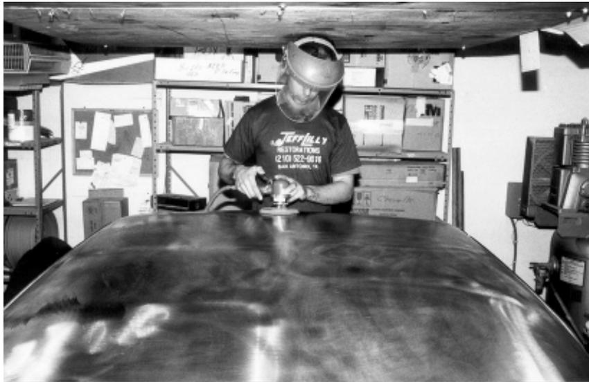
13. Before priming the steel needs to be sanded smooth and acid prepped. National Detroit DA with 80 grit scuffs the surface super- clean and smooths it to the right level for acid cleaning.
