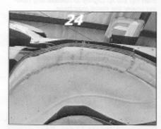
From the ground looking up, this is the inner wheelhouse welded in place. It's easier to do before the quarter is permanently attached. Lilly used a Mig welder.
