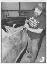
Tape off your existing quarter panel at the very top, two inches outward from the crown of the quarter or Bel Air moulding holes. Do this from the end of the taillin
