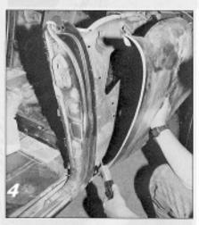
Cut along the edge of the quarter to the outside of the panel as shown. You want to leave some of the old panel to allow for the fitting of the new panel.
