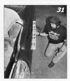
As you can see, our quarter is straight and flat just the way the Bow Busters ordered. If yours is stubborn and wants to come back when tension is released, you may need to massage the panel a bit. Try pulling the quarter back out. While tension is applied, take a slapping spoon and a body hammer; use a torch to lightly heat the wheelwell lip, then tap the lip slightly to release any holding power the metal may have.
