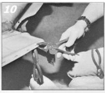
To be factory correct you'll need to install the rubber seal and support strip with staples. We use Blue Point .051 soft stainless steel wire from Snappon, preferably using an automatic center-punch mark every half inch in the middle of the flange. Then, using a .052 drill bit, drill holes in all marked flanges and deburr all holes. Start with an eight-inch-
