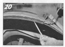
Place a 3/8-inch rope in the groove of the rubber, then pull the rope out after you fit and permanently weld the quarter. This will flap the rubber and seal up as per the factory technique. You will also need to install a new seal to the support side
