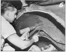
Once the outer quarter panel has been removed, you'll need to scrape the undercoat from the inner wheelhouse and check for rust damage. Use a 1300 degree heat gun and stiff putt knife.
