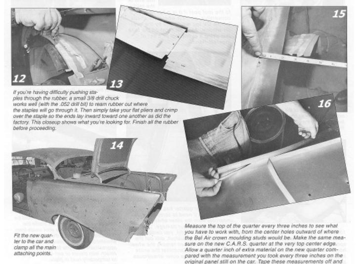
cut right on the line from tailfin to roof post.
