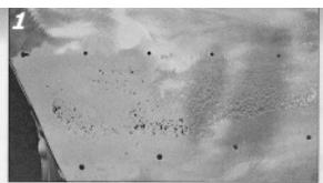
There are many other reasons for replacing a quarter. Excessive rustout under the Bel Air aluminum side frim is another problem, created by moisture held by the factory caulk adhesive used to hold the trim tight and squeakproof. Your first step is to remove all the mouldings, side, upper and rear stainless trim and taillight housings and bumper.
