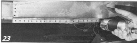
Using a hole puncher or drill, place holes at the very bottom of the quarter to the rocker panel, around the tailfin and all flanged edges. These will be used to weld the panel to the car's flanged edges.
