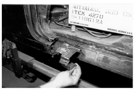
24. Here is the outside rocker panel end piece being pulled free once you cut the spot welds. This piece cannot come out until the center section of outside rocker is removed.
