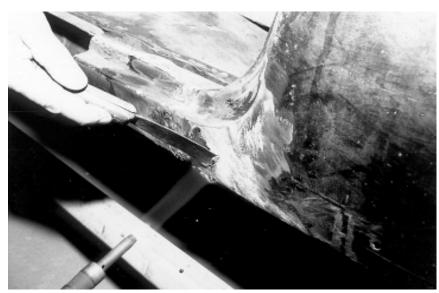
16. Located just below the back of the door is a lead seam. Heat the lead and scrape it with a putty knife. Take the wire brush on a drill and brush the remaining solder out so you can see the seam where the original factory rocker goes inside the edge of the quarter panel.
