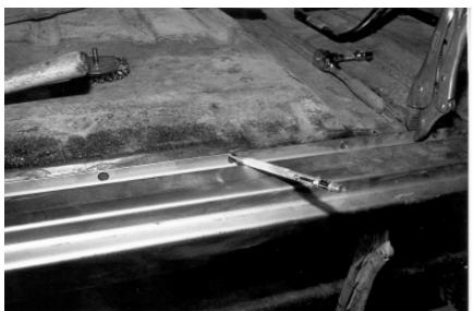
57. This photo shows the top edges of the floor and rocker, where they mate in place with the door open.
