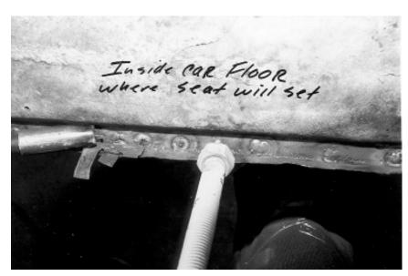
39. Use the panel holder on the floor edge. Start in the center and work your way out toward the front and rear of the car.
