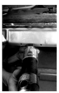
48. Take a flanging tool that has a pneumatic hole puncher and punch-out holes in the bottom rocker to weld the outside rocker to the inside rocker. You can also use your drill and SpotEze and drill out appropriate holes.
