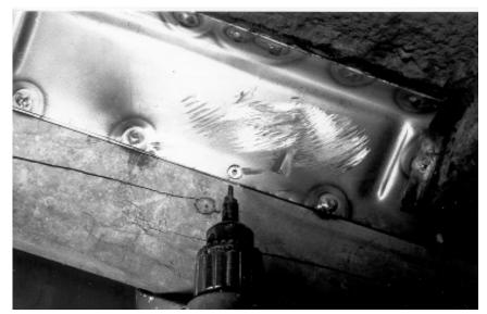
56. Another method of doing the bottom edge of the rocker, is to make sure that the two pieces of metal meet up for a good fit. Drill through one panel only and then weld the two together. Use vise grips to clamp the edges together when welding from floor. This photo is from the under-car backside view of the inside rocker.
