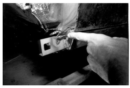
66. Weld it in the original place where you drilled out the spot welds. Fill with weld to attach solidly. Now if you want to replace just a small section of a rocker that might have a hole and you want it to be authentic then proceed to the next booklet (Partial Inside Rocker Replacement)
