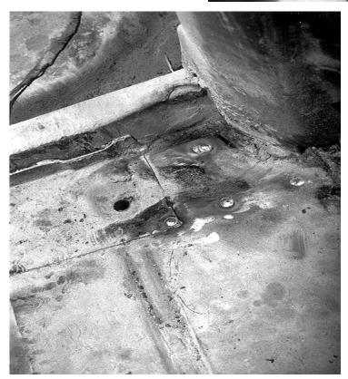
$45. \ \mbox{This}$  photo shows the completed welds inside of the brace on the floor.
