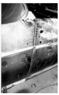
33. Shut the door and check the gap. If the gap is satisfactory, then proceed. If not, then use a floor jack and 2X4 to support six inches to one foot on rear brace behind where the door and quarter meet. Jack it up to the correct gap, hold it there and then proceed.
