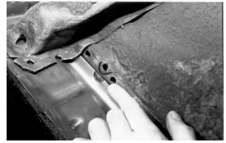
35. Line up the new inside rocker with the original half moon notch that was left from years of rust discoloration. This picture shows where the rear brace meets up with the inside rocker. You need to push it up into place so it fits.
