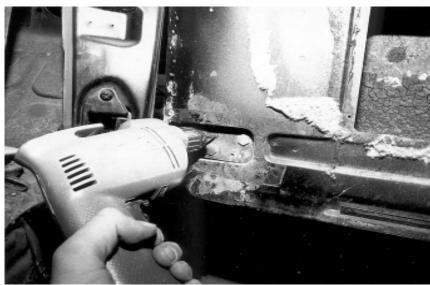
9. This brace is mounted to the center body mount to keep the body from sagging because we are performing this restoration with the body off the frame . If the body is still on frame you'll be able to perform this restoration but it is much more time efficient when the body has been removed from the frame. This brace can be shimmed to adjust door gap if body sags slightly. Be sure and install two braces one on each side.
