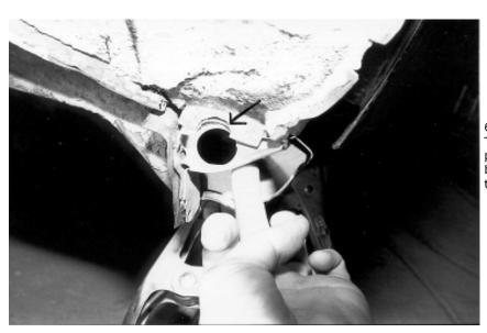
63. Now take the inside access plug bracket. The arrow points to the three flaps. The pillar post, the rocker, and the flap of the plug bracket. Make sure these all lineup close. Hold them in place and tack weld it in the corners.
