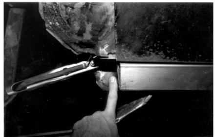
53. The edge needs to be lined up with the front fender and rocker. (Check that the edge of the door lines up with edge of rocker)
