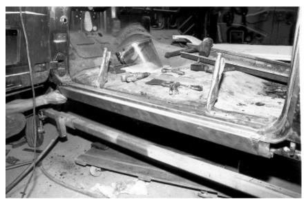
51. Position outside rocker in place. Here you see how it slips back in once you have cut the groove mark in the last step.
