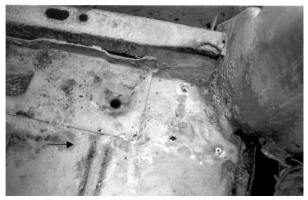
29. At this point if your cars body is still mounted to the frame Take a floor jack with a 2X4 and jack up 1/4 inch clearance between brace and frame and remove the brace. This needs to be removed to replace the inside rockers regardless if body is still on frame or not. This is the brace you just drilled out where your feet would go in the back seat.
