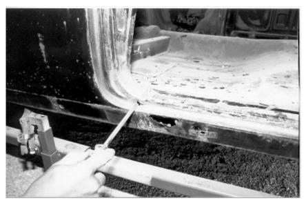
2. This is a close up of a typical area where the rocker is rusted out leaving holes under where the rocker moulding would be..
