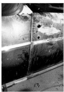
7. Before you go farther check that the door gap lines up correctly: a good 3/16 to 1/4 max gap all the way around the bottom of the rocker, the quarter and the fender. (if the gap is not right, make sure you line it up right before you proceed)
