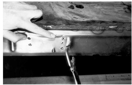
41. Now go to the other side of rocker and use the Spot Eze on the pilot holes. Cut through the rocker and stop when you hit the floor brace.
