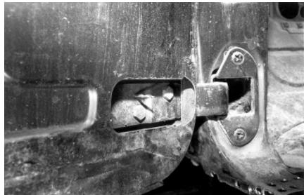
32. Put your door back on the car. Line it up and put in the 1/8 drill bit guide pins. It should line up perfectly.
