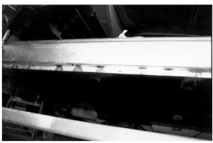
60. You can see here that the welds have been made approximately 2 1/2 inches in between on the underneath rocker.
