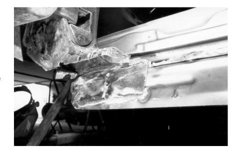
47. Take the plate that connects to the bottom support that you cut before in caption # 27. Now place it over the inside rocker in place and weld it in solid.
