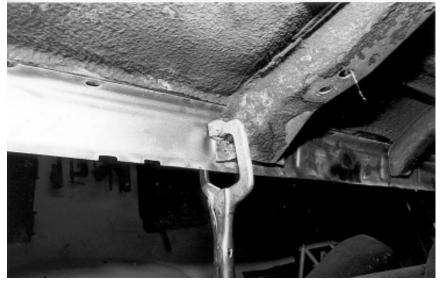
38. Here is a home made panel holder that uses a threaded rod with a pad on top to butt up against your shoulder.
