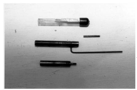
10. This is the Spot Eze tool with replaceable center drills for cutting factory spot welds out. Drill out every weld in areas described. Blair circle or cookie cutter spot weld tools work just as good.
