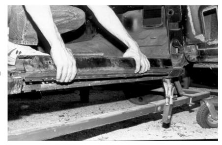
20. Get inside the car. Pull the rocker up and down to loosen and remove rocker. If it still will not come free you may have missed a spot weld somewhere.
