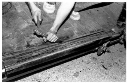
18. Take a heavy duty flat chisel or putty knife tap it in easily to loosen the panel. Be careful not to bend the edge of floor.
