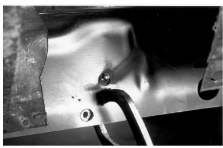
42. Now weld starting at 12 o'clock position going around clock wise till completely welded solid. This will join the rocker and brace.
