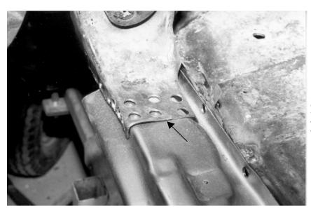
54. Open the door and make sure that the edge below bottom hinge goes up and fits flush, that the rocker makes good contact with the floor where you see the six spot welds. See arrows.
