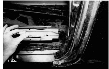
50. Take the outside rocker and lay it down. Take a marker and mark a straight line where you will need a groove to slide it into place. Use a 3/32 cut off wheel and make a groove.
