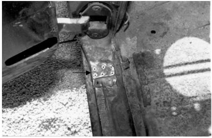
15. At the end of the door just inside of the rocker where the quarter panel starts, there has been some slag weld that was welded on from a previous repair. Normally the spot welds would be in the center of this piece just like the front one. Clean this with the wire brush and drill them out.
