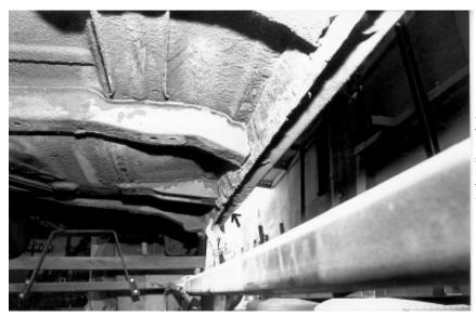
4. This is the opposite side of the car. Notice the arrow pointing to a wrinkle where it had been damaged at one time. This complete inside rocker needs to be replaced. More than likely someone used a floor jack to change a tire and placed it on the rocker instead of the frame.
