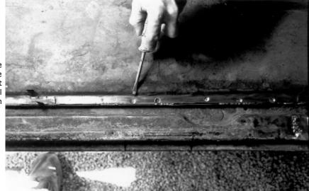
12. In this photo you can see how some of the spot welds have been drilled with the Spot Eze and some have not, so that you know what it should look like. Drill through one layer of steel only. Which will separate the floor panel from the inner rocker top edge.
