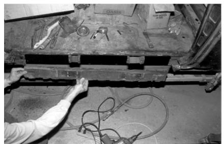
23. Cut each end of the inside rocker and pull it free. Notice the floor braces still in place.
