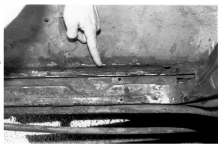
6. Right under the same groove as mentioned in caption #5 (the rear seat), scrape out the body seam sealer with a putty knife.
