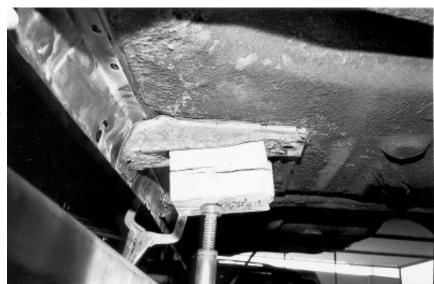
44. Take the floor brace you took off the car and get it into position, use a piece of wood and a bottle jack. Adjust until flush. Weld rocker to brace first.
