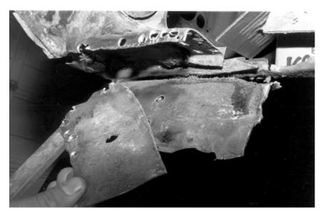
27. After you remove the front section there is a plate that rides over the top of the inside rocker, slice this plate with a cut-off wheel, out of the way ( keep it. ) This is much faster than removing the whole plate which goes up into the car two foot.
