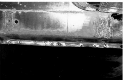
13. The bottom flange where the inside and outside rockers meet below at the lowest point of the rockers (repeat the process of finding spot welds and drilling them out with the SpotEze
