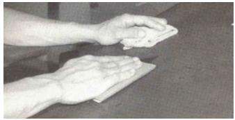
This is the proper technique for colorsanding. Hold the block flat and always have a damp, clean cloth nearby to keep the work area wet so that the paint will not build up on the paper. Check your paper every 20-30 strokes for buildup. When you see small traces of paint or clear sticking to the surface, turn to a new side or get a new sheet. Determine how many strokes it will take to ,remove any orange peel and try to use that same count on the rest of the body.
