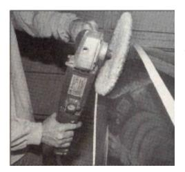
You will need a variable-speed electric buffer with a range of 0-3,000 rpm for proper buffing. It should be set between the 1,800and 2,300-rpm mark for the best effectiveness. At any time you can change the speed to get into small areas.
