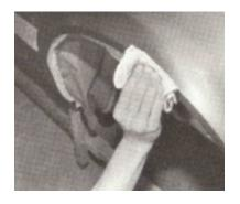
Here is the edge of the wheelwell being polished by hand. Four fingers together work well. Then take a clean polishing cloth and buff out the area to a high shine while removing any remnants of compound sludge.
