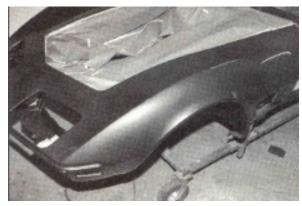
The wheel wells should be masked so that the underside isn't contaminated.
