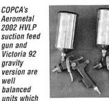
feature a Teflon cup on the suction feed, stainless steel internals, anodized bodies for quick clean up and are available with a full range of tip sizes and a built-in air regulator. Each gun comes with a maintenance kit which includes lubricant, brush, wrenches, seals etc. These guns also can double as a primer/paint gun.
